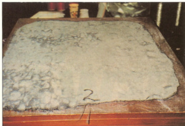
Figure 5: The slit tape woven sample on a backlighting inspection table. There are no signs of imperfections that would lead to any loss in hydraulic properties.
