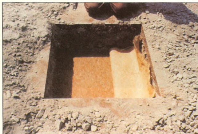
Figure 6: Slit tape woven fabric being exhumed from location 3.
