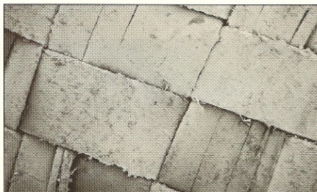
Figure 15: Slit tape woven fabric illustrated in a scanned electron microscope photomicrograph.
