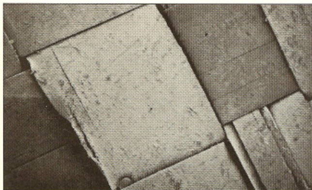
Figure 14: Slit tape woven fabric exhumed from location 3.
